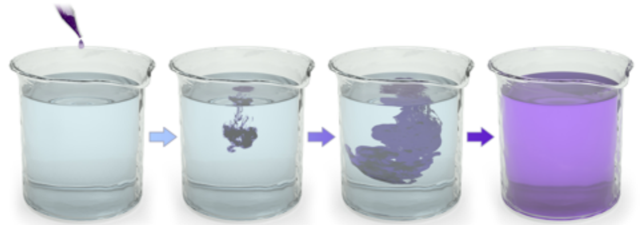
Diffusion of particles due to a concentration gradient
