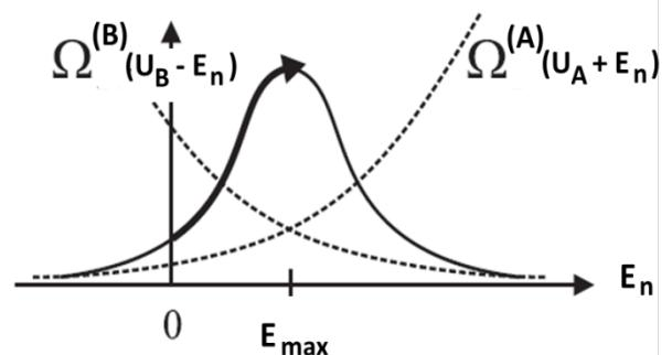
Exchange energy until entropy is maximal
